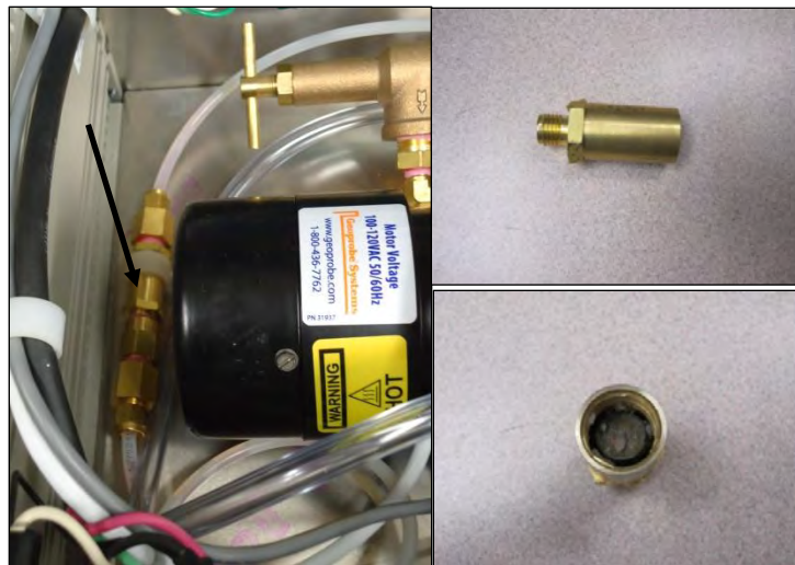
Figure 7.2: Location of Inline Filter in K6300 and buildup of particulates in filter.
