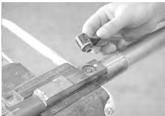
Figure 8.1: Unthread the membrane from the probe block.
